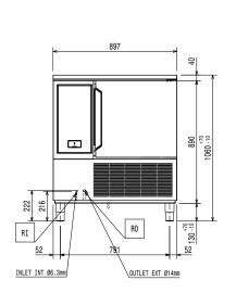
Drain Electrical inlet (power) ΕI Refrigerant Outlet
